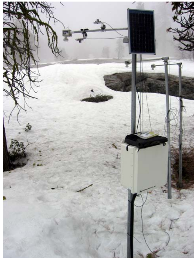
Photo 5. Close up of acoustic snow-depth sensors, with up-looking and down-looking radiation measurements on nearest sensor arm, Southern Sierra CZO.
