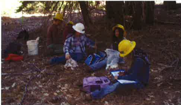
Figure 3. Nitrogen deposition from the atmosphere to the ground and movement from the ground into the mineral soil is measured each year with resin lysimeters (shown in plastic bag in photo foreground) at hundreds of points across the watersheds. This photo shows a team of Sierra High School students installing resin lysimeters at a Providence watershed in 2012. Photo: C. Hunsaker
