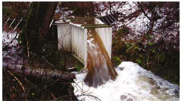
Figure 4. Fiberglass flumes provide a uniform stream cross-section for accurate stream discharge measurements. This photo shows high flow at a Providence Site stream during a rain-on-snow event that created stream turbidity (suspended sediment) which is measured at KREW. Photo: T. Whitaker
